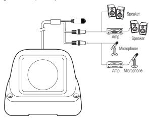
1. Connect the AUDIO IN port of the camera with the microphone or LINE OUT port of the amplifier that the microphone is connected to.
