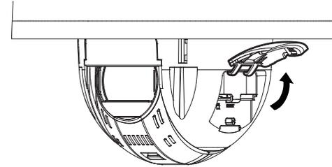
3. Insert Micro SD cards in the direction of the arrows as shown in the figure.
