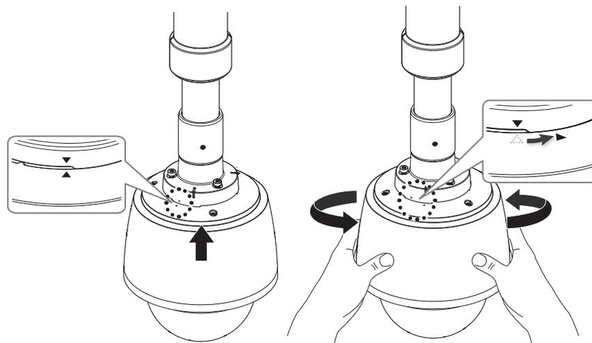
6. Tightly fasten the 3 mounting screws on the top side of the mount.
