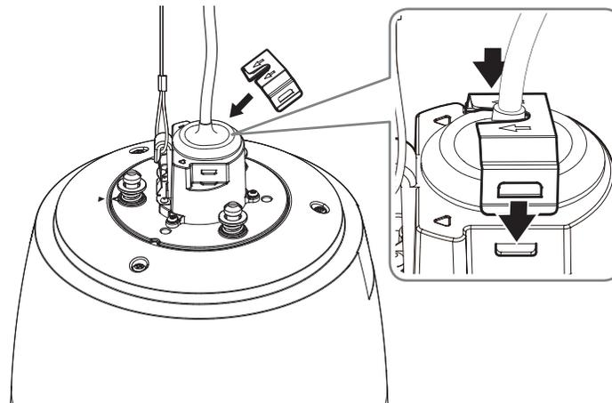
5. After aligning the installation direction guides of the camera and wall & pole mount, push the main cover upward and turn it counterclockwise until it is secured.
