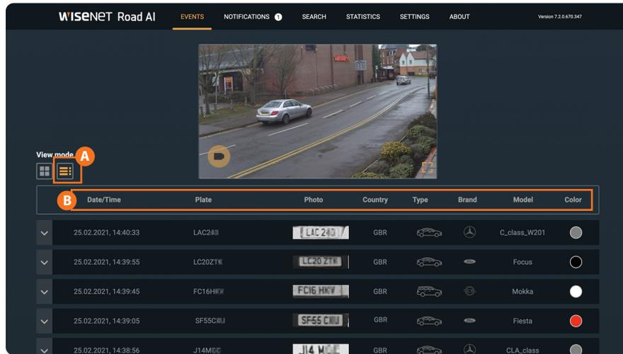
To enable the list display of events, click on the **A** corresponding button. Such event parameters **B** as **Date/Time**, **Plate**, **Photo**, **Country**, **Type**, **Brand**, **Model** and **Color** are displayed as a table. The events are displayed in a list from the newest to the oldest.
