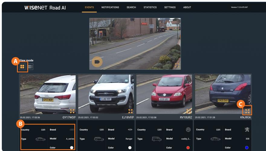
To enable the display of events as a table, click on the **A** corresponding button. In this mode events and their parameters (**Date/Time, Plate, Direction, Photo, Country, Type, Brand, Model** и **Color**) are displayed in blocks.
