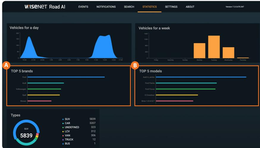
**A** The **Top-5 brands widget** shows the car brands statistics based on their statistical distribution (no more than 10,000 latest cars are taken into account, due to the limitation of the database size).
