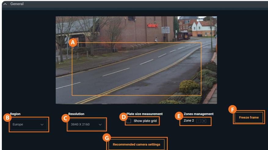
**A** The application settings allow the user to move the or resize the frame within which the reading takes place.
