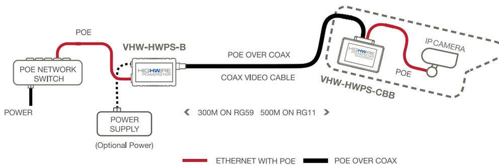
HIGHWIRE Powerstar Backbox delivers Ethernet and POE over legacy coax, for maximum reliability without re-wiring.
