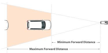
Camera in 4K mode can cover up to 3 road lanes. The FullHD mode can cover up to 2 lanes.
