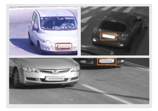
Too much light. Either adjust the iris or shutter speed. Night time: dim the IR or set AGC to Low.
