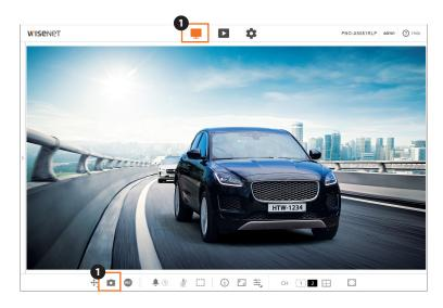
2 Use Plate Grid tool in the Settings tab of WisenetRoadAl and Freeze Frame feature to check whether plate fits the allowed range.
