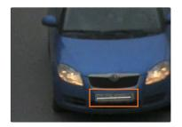
Improper focus settings. Adjust the lens.
