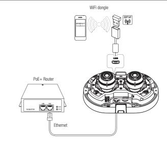
The Micro USB port of the product is provided for easier installation, and is not recommended for monitoring purposes.
