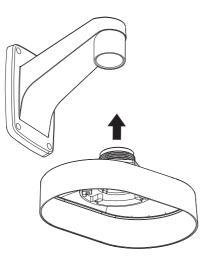
3-2. Attach the mounting plate to the hanging mount using the appropriate screws.
