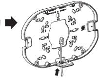
1-3. Pull out network cable through the hole in the mount plate.
