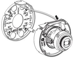
9-1 • Installing network cable (PoE)
