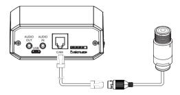
= Turn off the camera power when connect or remove lens module.
