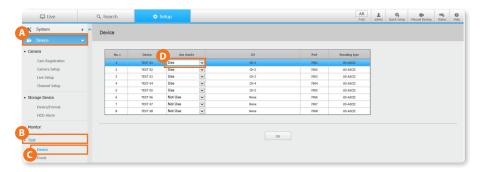
Check the NVR settings to obtain corresponding Port number in (A) Device → B Text → C Device setting (by default port 7001 for CH 1, 7002 for CH 2, etc.)
