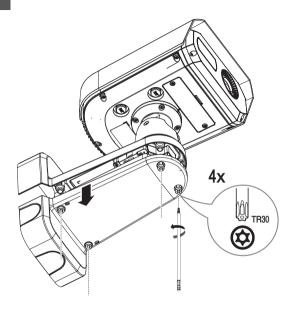
2-1-1 • When installing on a wall
