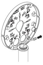
10-1 • Installing network/power cables
