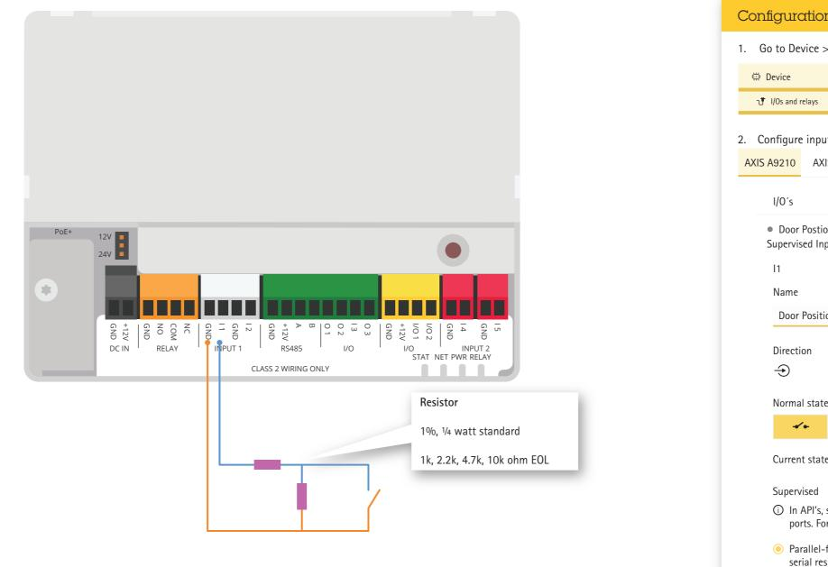
Adhere to local life safety code in all installations. Illustration does not depict door monitors, REX devices, locks, controller power supply, network switch, battery backup and UPS. Ensure that your power supplies and relays are rated for the intended purposes. This is just an example. Please refer to product datasheet for details and the device's web interface for power states
