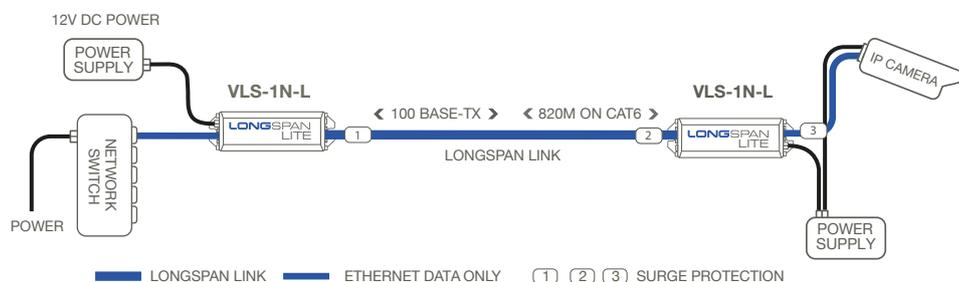
Range is for typical 24AWG Cat5e or 23AWG Cat6, 4-pair UTP. For other cable types, or any installations over 600 metres length, consult Veracity for recommendations or test on site.
