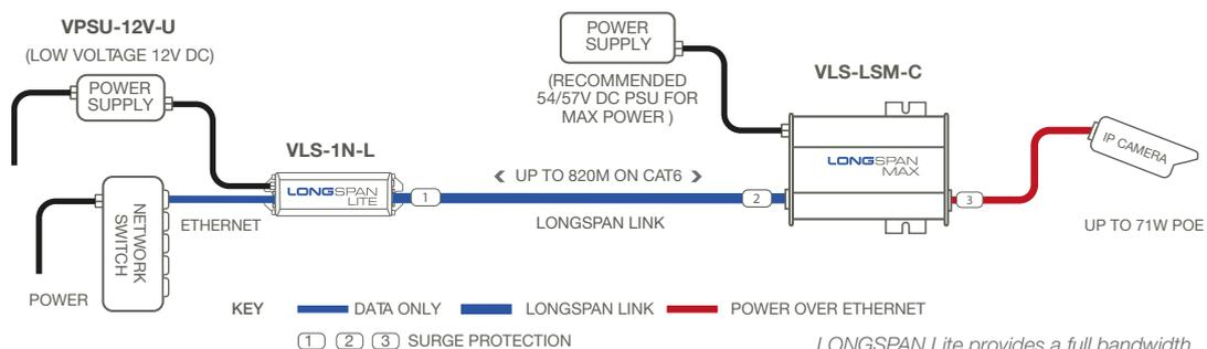
LONGSPAN Lite provides a full bandwidth link to a LONGSPAN Max Camera, locally powered for maximum POE output to the IP camera.
